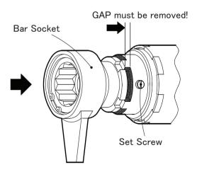
O Pull the bar socket in order to confirm that the bar socket was mounted on the wrench body completely.
